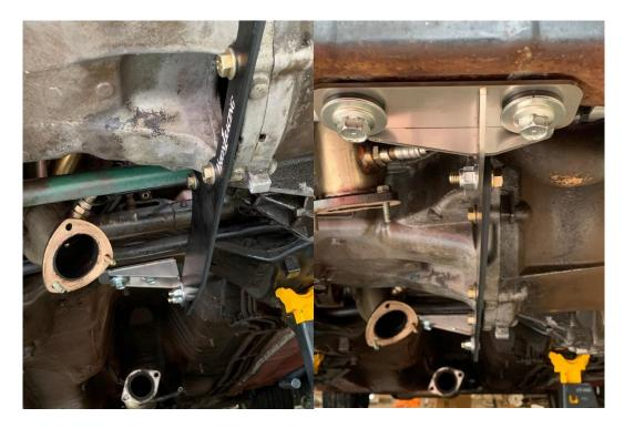
Leaving the bolts slightly loose at this point is a good idea to aid final assembly
